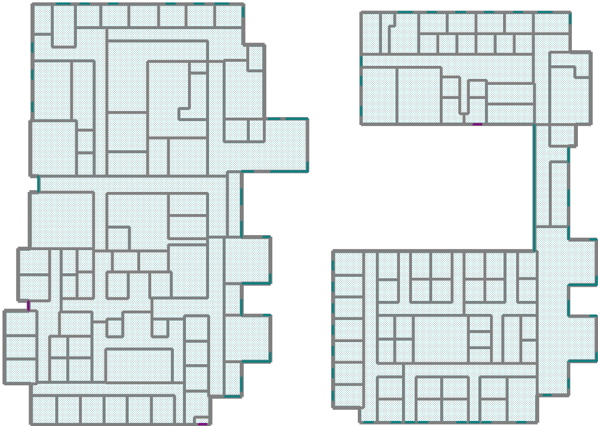
Figure 2 – 1 st Floor zoning/floorplan of eQUEST model
