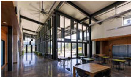
Radiant slab and ceiling fans provide the building's heating and cooling. - Photo Credit: Stephen Miller
