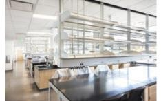
The research lab areas are laid out in open modules to allow for flexibility in usage by different researchers with differently scaled projects over time. The bench layout is perpendicular to the exterior windows to maximize daylighting penetration. -
