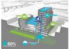
The north wing upper roof and atrium rooftop serve as water collectors for the rainwater reuse system, while the south wing and lower roof on the north wing provide habitat for native species. - Photo Credit: SERA Architects
