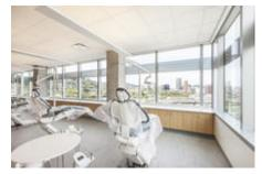
Recognizing the importance of natural light and its link to productivity and health, the design team strove to daylight all regularly occupied spaces, while mitigating heat gain, by providing filtered light through shades attached to window mullions located above the view area. - Photo Credit: Alene Davis Photography
