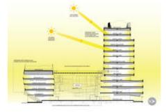
The narrow footprints of the north tower and south bar allow for ample daylighting; where the two masses engage the central atrium space, daylighting is borrowed from the atrium using interior glazed walls. - Photo Credit:
