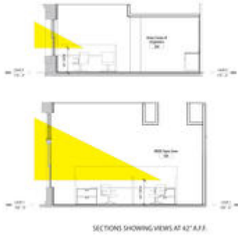
Sections showing views at 42” A.F.F. - Photo Credit: Design- Build Partners: The Beck Group and Westlake Reed Leskosky
